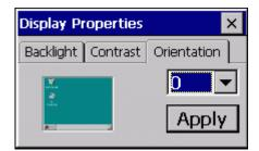
Display orientation can be set with the «0» (default setting) or «90» settings. The display is rotated in a clockwise direction. The «90» setting should be selected for vertical mounting. The picture on the left of the dialog shows the orientation set. The setting is not transferred until after a restart.
